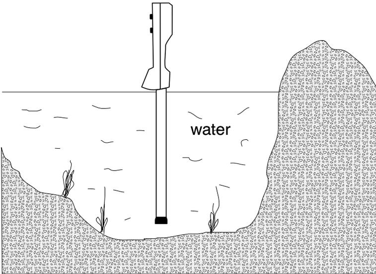
Hold the locator in a vertical position while searching to produce the best results.
