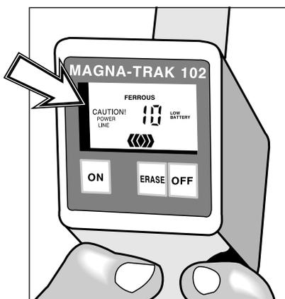
The distance or detection range from the cables where the locator responds depends on the energy being carried by the electrical conductors. The higher the energy, the greater the distance the locator will respond to it. If the cables are dead (no electrical connection or energy transfer), then no visual indication will appear.
